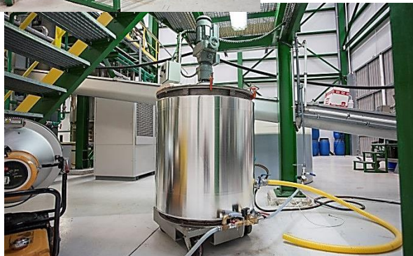
CENER High solids enzymatic hydrolysis 200L stirred tank reactor
